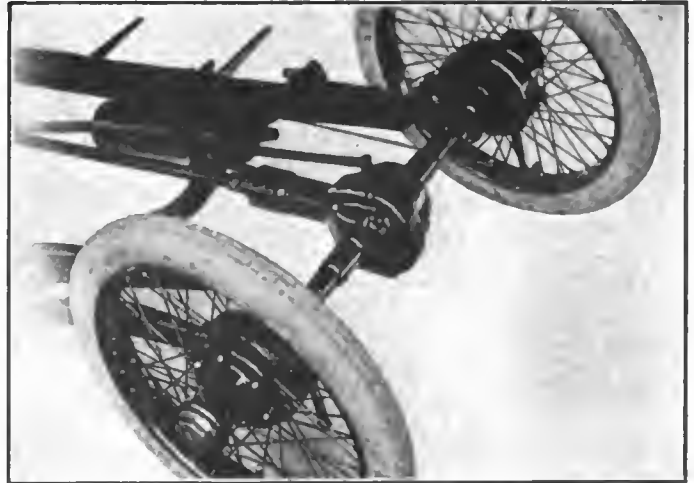
Rear construction of the Scripps-Booth showing the cantilever spring supporting the rear ends of frame, mounting of muffer, etc.
